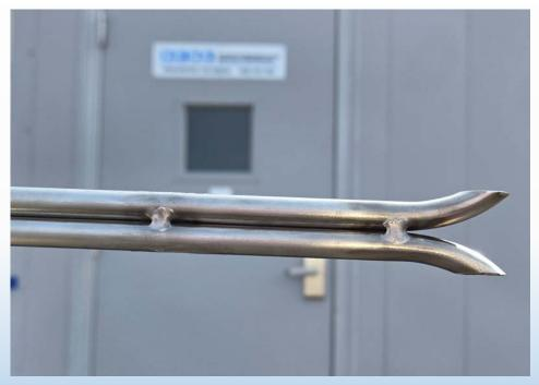
• Temperature is measured along with DP to be used in the calculation of velocity and to standardize measurement.
